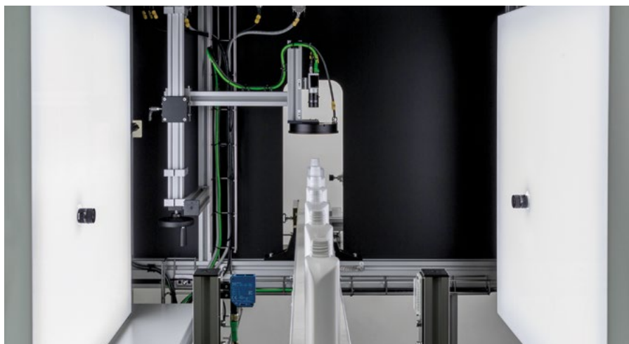
Bottle inspection system covering all fundamental and most common defects
