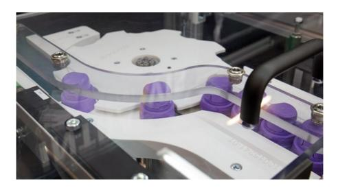
cially adapted to your space conditions and your inspection needs for your closure. Even a space-neutral integration can be realized. On the other hand, you get the guarantee that typical defects in the hinges or joints, which commonly occur in the production of specialty closures, will be reliably detected and sorted out. We can draw upon more than 10 years of experience in the specialty closures market.
