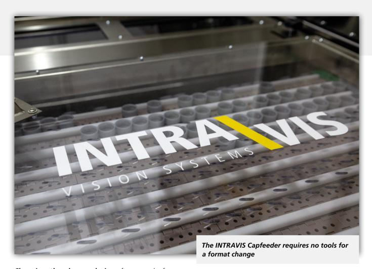
Changing the closure design, for example from PCO1810 to PCO1881, can be done without tools and in just a few steps. Even larger format changes, such as from 26mm to 38mm, can be carried out in no time at all. The subsequent validation of your inspection system can be carried out quickly and easily thanks to the convenient infeed of the appropriate test parts.
