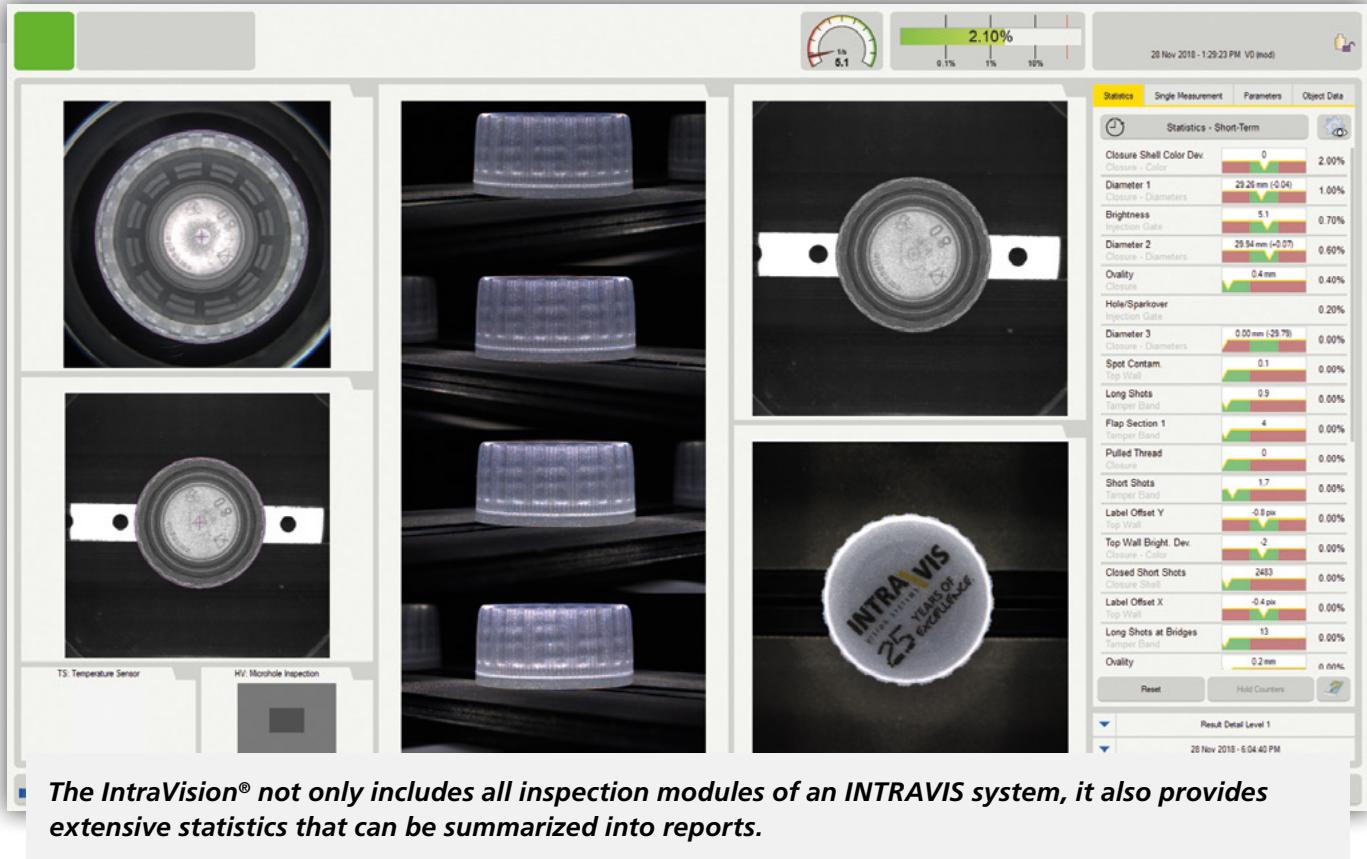
**IntraVision® is the inspection and administration software** for every INTRAVIS system. Embedded in it are the various inspection modules that are used to analyze parameters that are important for the customer product. But the IntraVision® offers more. The software **supports with important tasks of your job**.
