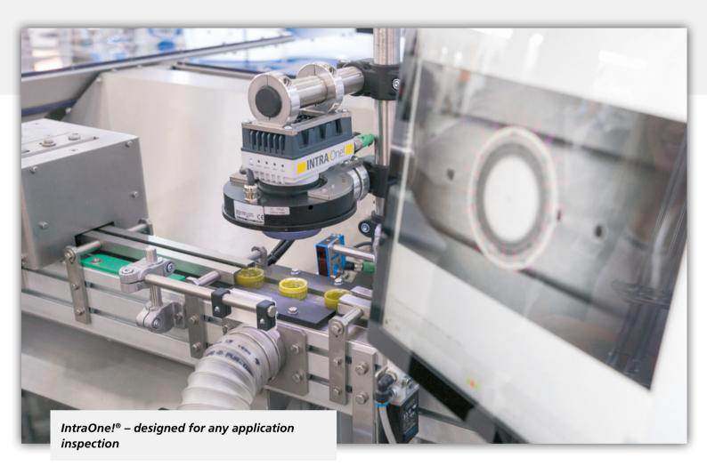
In addition to the basic package consisting of a camera and appropriate lighting for any inspection task, many options are available.
