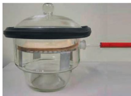
Fig. 1: Experimental set-up for artificial aging experiments and sampling with SPME. Glass desiccator with sample and lock for SPME fibre support.
