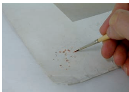
Fig. 5: Local application of potassium permanganate (0.5%) by brush for treatment of mould stain.
