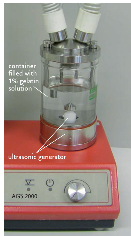
Fig. 6: The water container of the AGS 2000 intended to transfer the ultrasound to a container filled with 1% gelatine solution to facilitate a smooth workflow.
