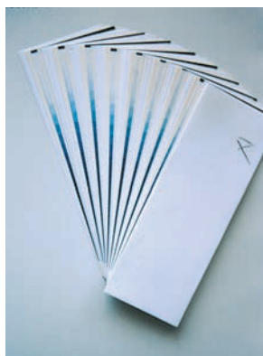
Fig. 1a: Each paper stack consisted of 8 standardised cyanotypes prepared on a pure filter paper (Whatman #1) sized with gelatin. Each cyanotype was covered with enclosure papers containing an alkaline loading on both sides. The enclosure papers were made of 100% bleached cellulose, containing different combinations of CaCO 3 loading and sizing agents.
