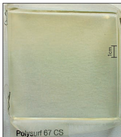
Fig. 2: Polysurf 67 CS™, 7%, poured into a polyester film mold, after 24 hours of swelling time.
