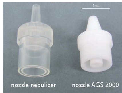
Fig. 5: On the left: the Nozzle of a Nebulizer that creates a regular aerosol stream; right: the nozzle of AGS 2000 ultrasonic mister that creates an aerosol stream shaped like a horseshoe.
