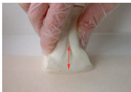
Fig. 7: Subsequent cleaning with a sponge soaked in a 2% Triton X-100™ solution.
