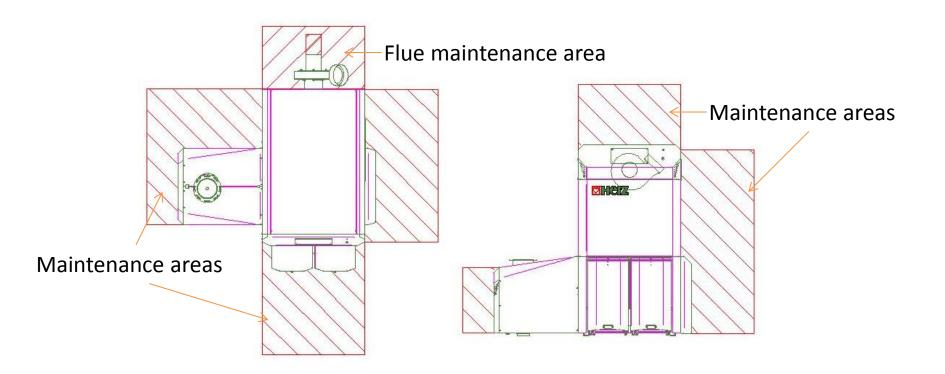
Required maintenance areas needed around a Herz biomass boiler are similar for most models
