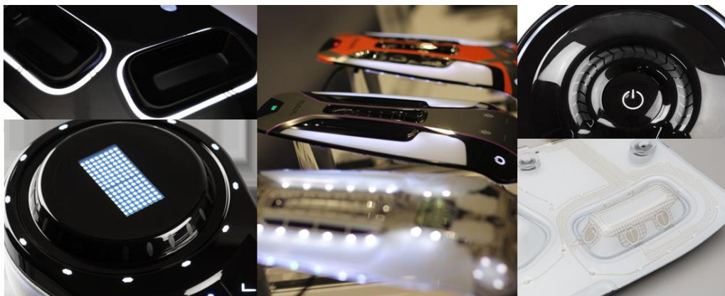
Fig. 4 The top-left photo shows a seat controller and bottom-right photo its electric film. Bottom-left photo shows a center console. The middle photo shows an overhead control panel. Top-right photo shows a technology demonstrator.
