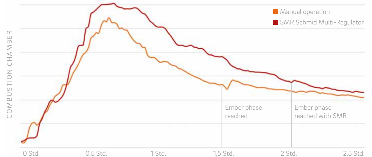
Comparison of two temperature curves, i.e. in the manual mode and with the Schmid Multi-Regulator. The point in time for adding fuel is reached later when the SMR is used and the average temperature is above that in the manual mode. With the regulator extended burning times are reached, i.e. less adding and improved utilisation of fuel.
