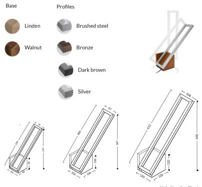
Unit of length millimetres (mm)
