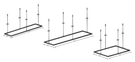
Unit of length millimetres (mm)
