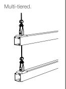
Maximum off axis suspension = 15° (unless otherwise specified by Gripple Technical Services)
